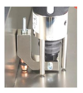
For welding of studs at a distance of up to 8.5mm To angled sheets
